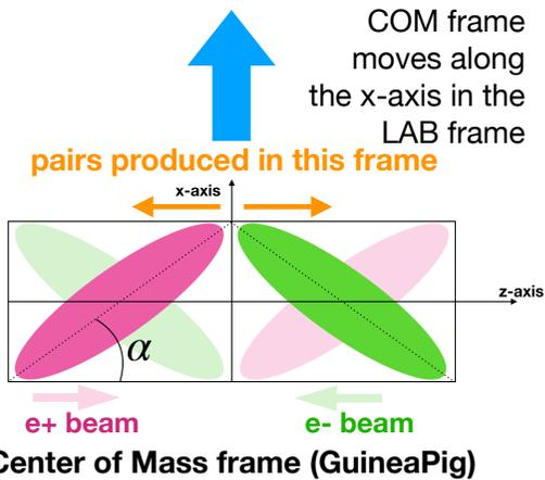
This process has been simulated using the generator **GuineaPig++**, which simulates the bunch crossing using a **step-by-step** approach to calculate the **EM-field** produced by the bunches for beam-beam effect.
