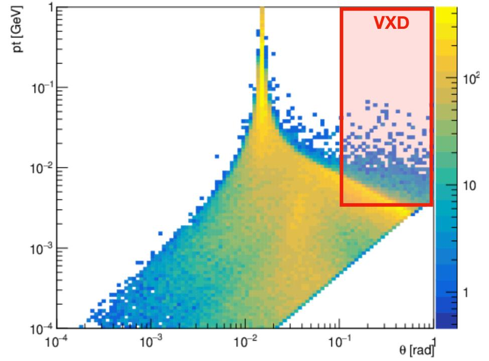
**Preliminary studies** on the occupancy due to the IPCs (generated with GuineaPig++ using the latest 4IP lattice beam parameters) show an increase of a **factor ~5** in particular in the **innermost layers** of the VXD barrel.
