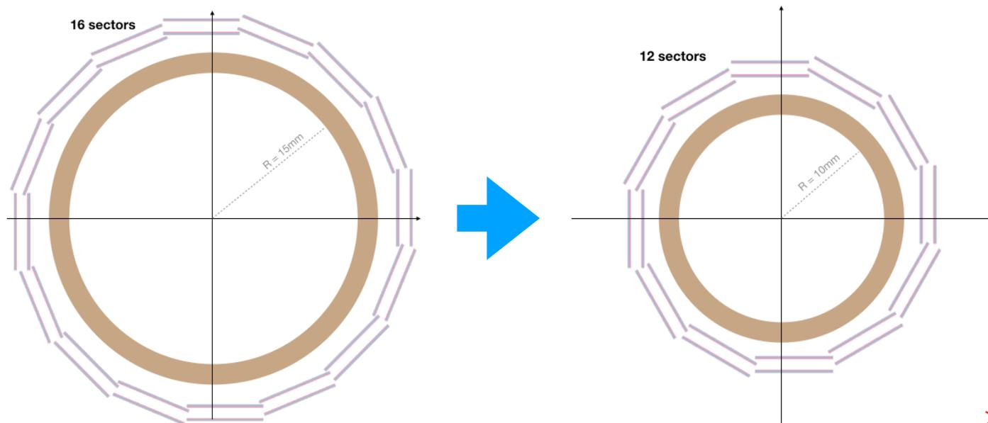
Also the **second layer** has been moved closer to the IP in order to have it **midway** between the two outermost layers.
