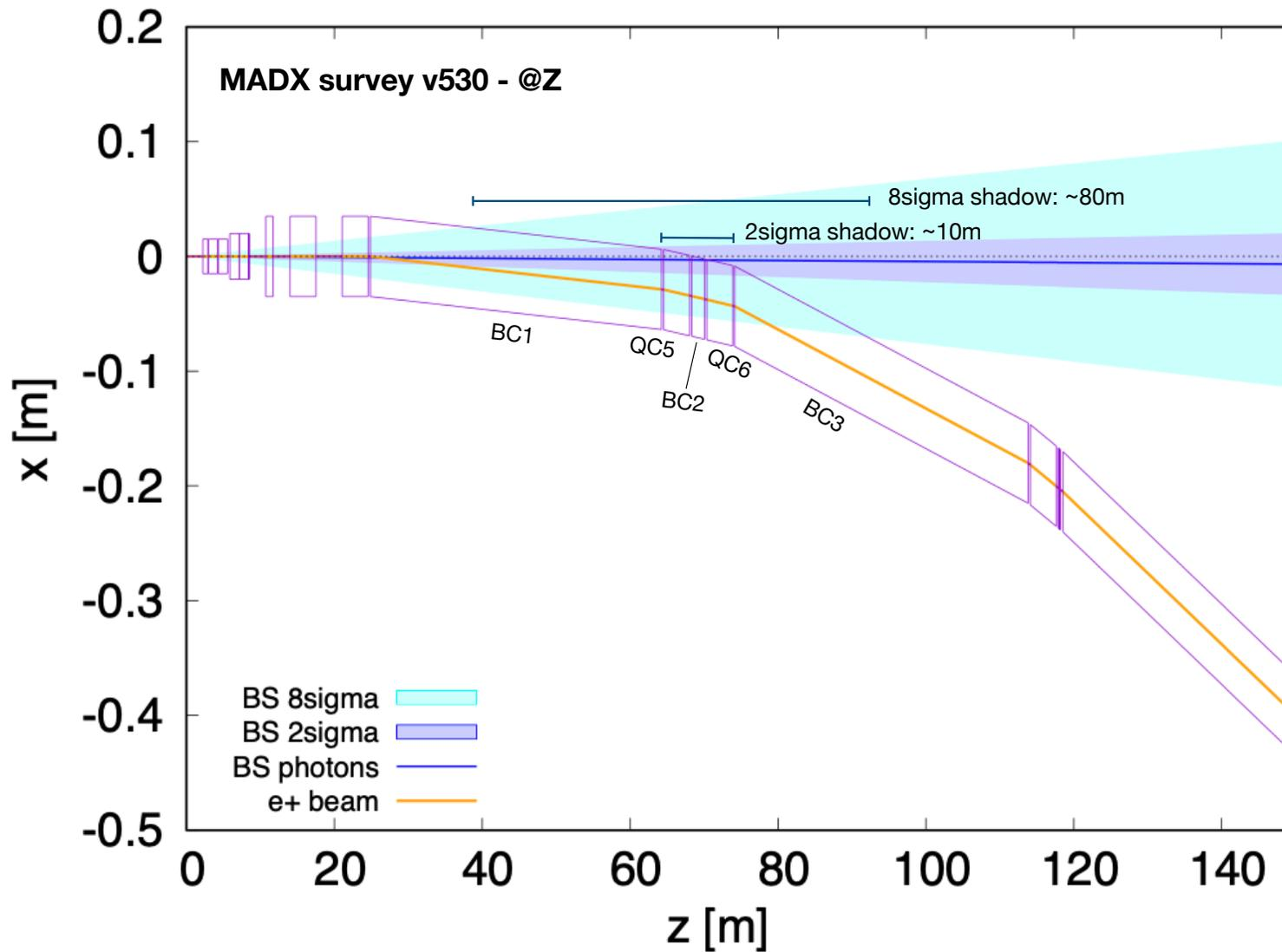
Comparison of the beamstrahlung photon distribution against the **MADX survey** for lattice **v530** show that the hits are localized in the “QC5-BC2-QC6” area - in agreement with the SR photons tracking in BDSIM (K. André 19/10).
