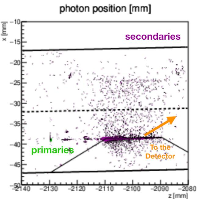
Main contribution comes from photons diffusing from the **tip of the Tantalum mask** which can end up in the detector region
