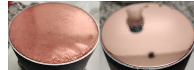
Cu QPR pre and post Plasma Electropolishing treatment
