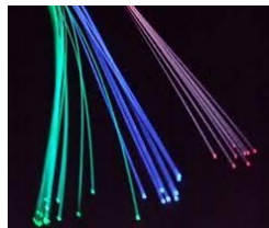
Plastic scintillator fiber (d = 1 mm)
