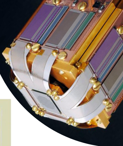
Topview of a detector design with sidecar geometry
