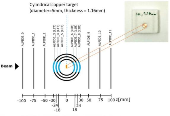
Telescope: 6REF (flat ALPIDEs) + 6DUT (bent ALPIDEs) + Target
