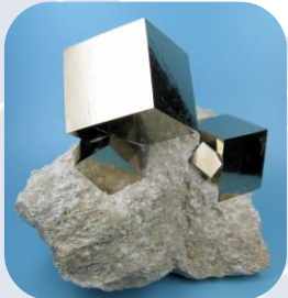
Examples of \text{FeS}_2 crystals with cubic lattices
