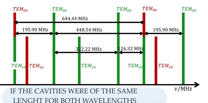
Simultaneous locking of the infrared and green light cavities at TEM00 was achieved when the green light frequency was shifted by 73 MHz.
