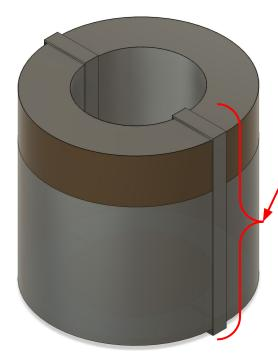
Long vertical Slit creates a parasitic capacitance
