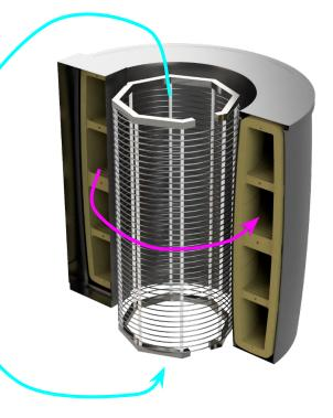
Flux is picked up by LC resonator
