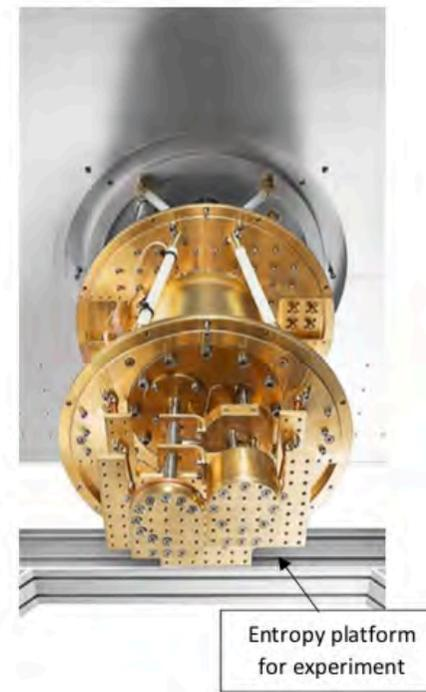
*cryostat open – with platform*
