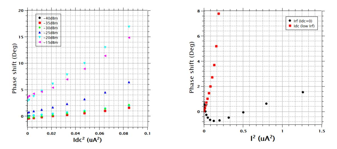
Nonlinearity is indeed on  $\sim \mu A$  scale !!
