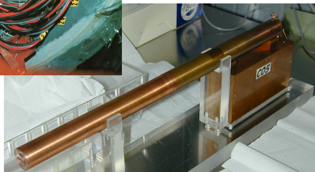
The counter shielded box, the counting shield hosting counters
