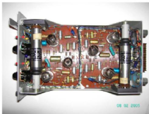
All real implementations of operational amplifiers will suffer from drift, non-zero input impedance and – most important – non-infinite gain. A gain less than  $\infty$  will yield (static) errors in computations so an amplifier suitable for an electronic analog computer will need a very large gain.
