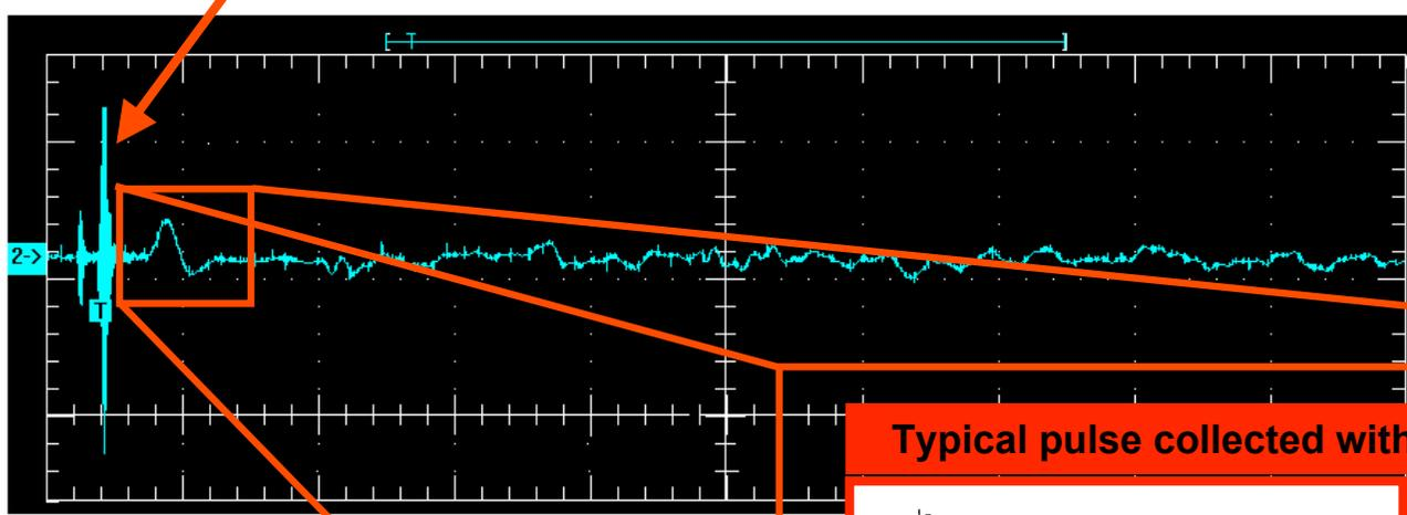
Typical pulse collected with  $\sim 10^{10}$  protons @ 200 MeV
