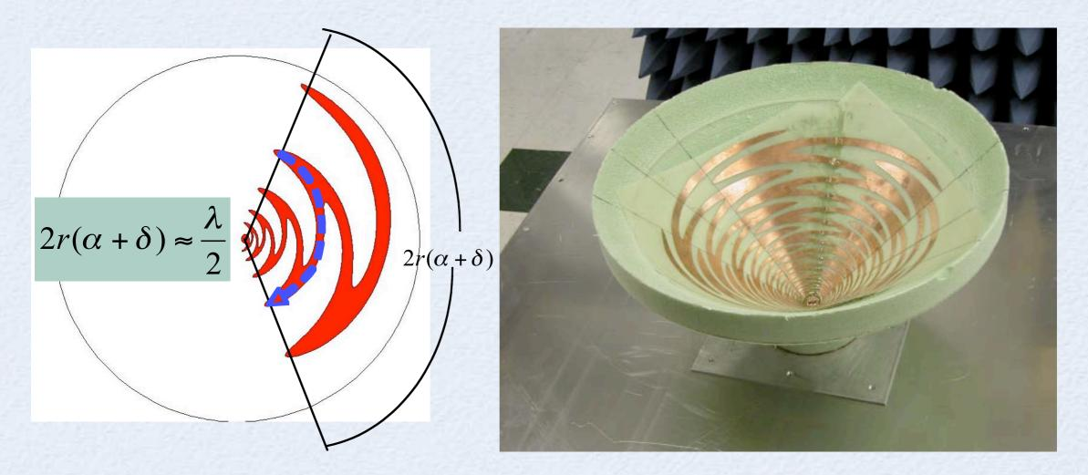
R. Bradley and Rohit Gawande tested FASR Feed (0.5 to 3.0 GHz) on 43m in May 2008 Cryogenically cooled feed by end of year.
