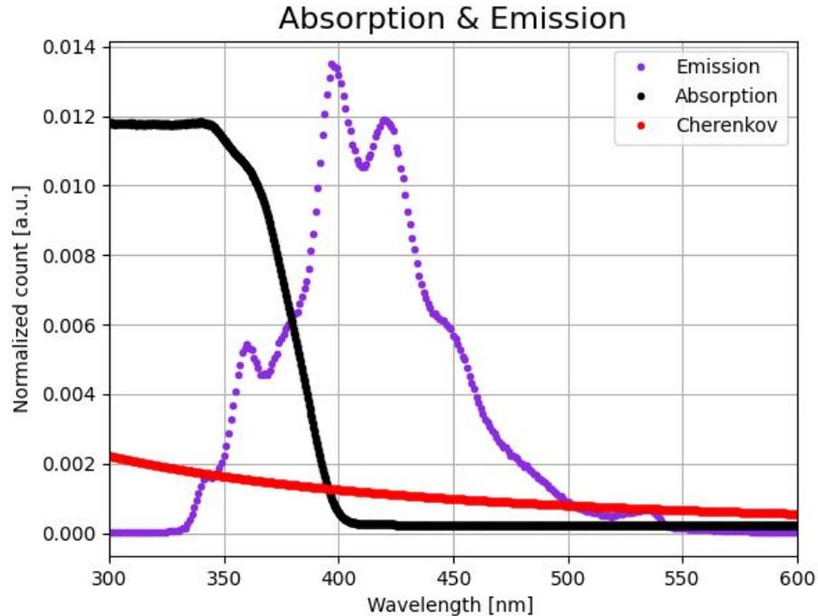
**Cherenkov light can be separated from scintillation light thanks to its spectral features.**
