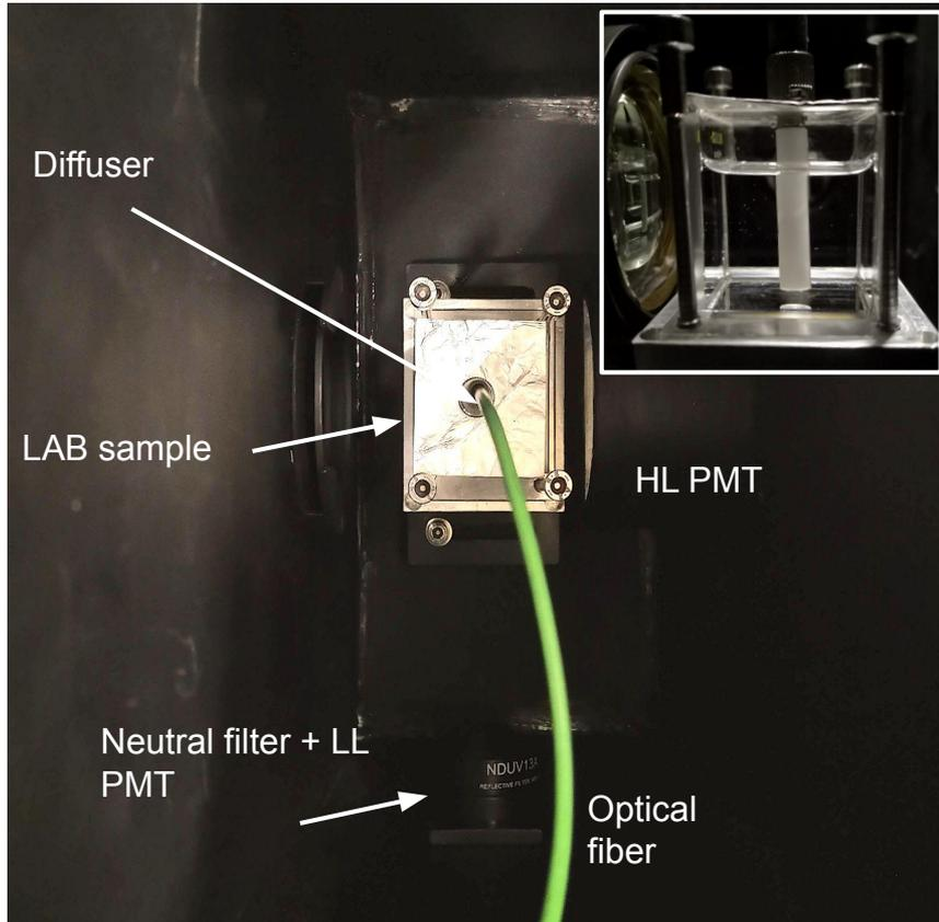
We used a **laser at 405 nm** to characterize the detector response
