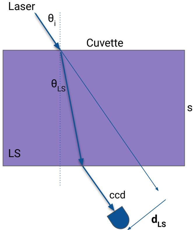
We used a **refractometer** to perform the measurements of the refractive index
