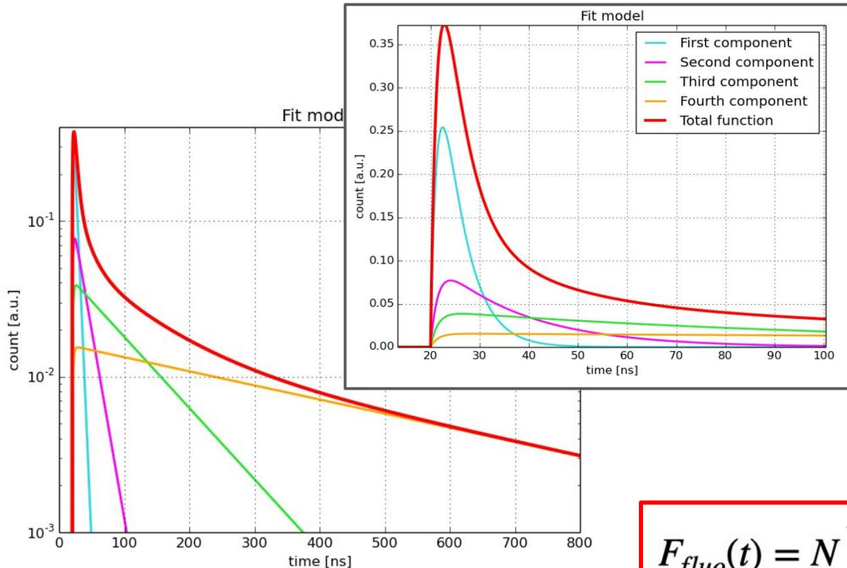
To describe the fluorescence time profile **4 components** are needed
