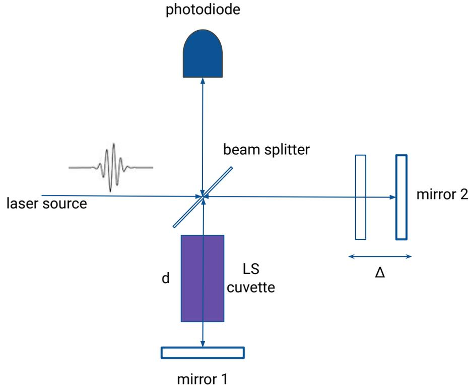
We used a **interferometer** to perform the measurements of the group velocity
