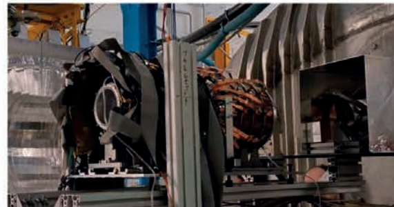
Figure 1: detail of the s122_2024 experimental setup. The KRAB detector is visible on the center along the beam direction. The DSSSD telescope (see text) is also visible inside the aluminium box on the right.
