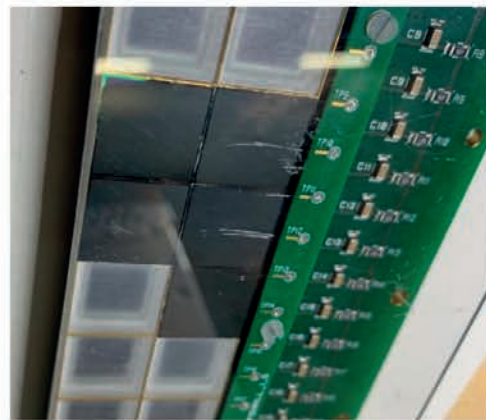
Figure 4: Picture of the long wire bondings between the SiC pads and the connection board pads.
