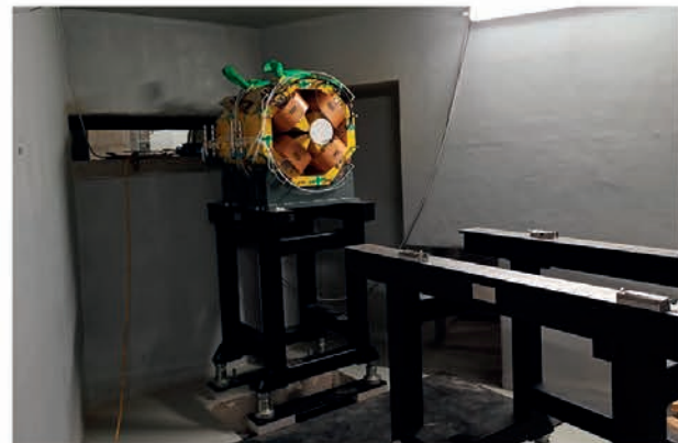
Figure 5: First quadrupole doublets on FRAISE room
