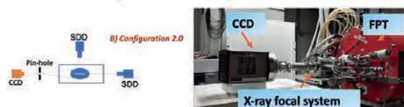
Figure 3: Pictures of the PYN-HO prototype operating in the second configuration for in-plasma measurements.
