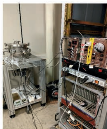
Figure 1: Test point with vacuum chamber and electronics at the INFN-LNS, used for the preliminary prototype qualification.
