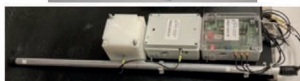
Figure 1. (Top) The developed WiFi front-end and data acquisition electronics. (Bottom) A monitoring unit consisting of one SiLiF and one SciFi detectors with their electronics.
