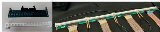
Figure 2. Top: PI3SO printed circuit board equipped with 16 SiPMs (top) and 16 CsI(Tl) crystal unit (bottom, white array) compose a module: four modules compose one linear array or detection unit. Bottom: one detection unit with four flanked modules, arranged for DAQ and characterization tests.
