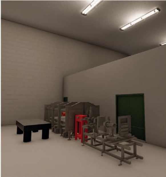
Figure 3: 3D rendering of the E1 area. The vacuum interaction chamber and part of the transport beamline for proton/ion beams are shown.
