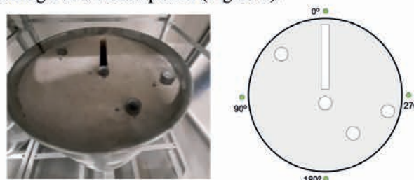
Figure 2. Top view of the mockup scheme; the four green circles (0°, 90°, 180°, 270°) indicate the position of the sensor units.
