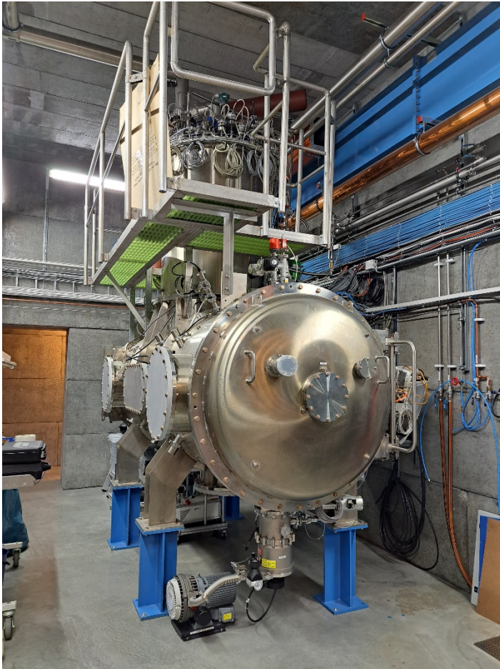
Figure 4- View of the HNOSS hirozontal cryostat (left) and of the CoW portable cryostat on wheels.
