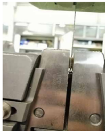
Force transfer system (welded ball and sliding tube) on the Nb 3 Sn strand.
