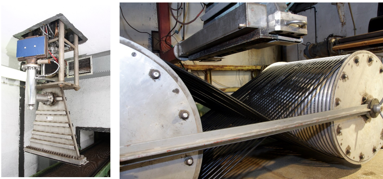
Figure 17 - View of the RAPID facility: (left) Elektronika 10-10 electron beam accelerator, (right) ILU-6 electron beam accelerator with wire crosslinking installation.
