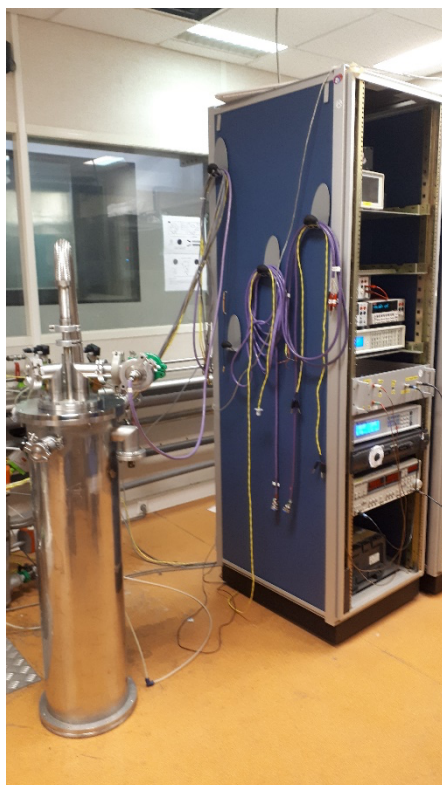
Figure 8 - View of the RRR facility at CEA
