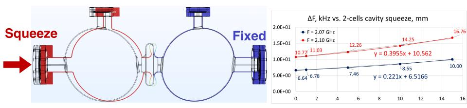
Now: leveraging the expertise of our incredible RF team to simulate coupled oscillators subject to mechanical vibrations (induced by GW or ambient noise) and derive expected growth rate of the signal mode due to parametric energy transfer from pump mode for the three pairs
