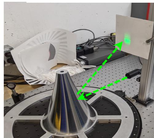
Measuring focal spot dispersion with laser
