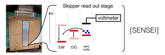
Skipper CCD: non-destructive charge measurements reduce noise
