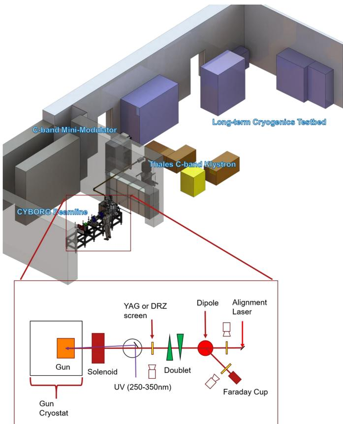
Multi-Objective Testing of High Gradient RF Accelerators (MOTHRA) laboratory and CYBORG beamline (above)
