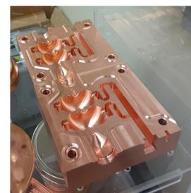
High power BDR test cavities (left); cathode coupling test (below)
