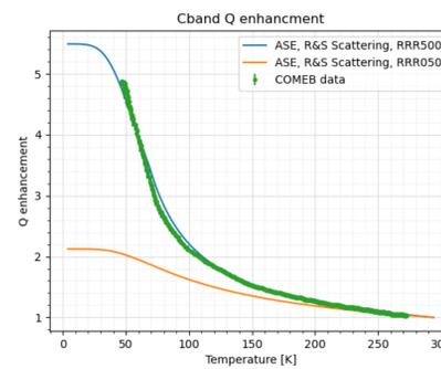
LLRF pillbox measurements of Q enhancement at cryogenic temperatures
