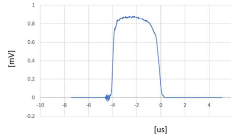
C-band klystron forward output from Thales tube with XK5 pulse tank and custom PFN. 5710 MHz central frequency (corresponding here to 500 kW)
