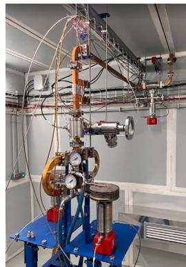
A) RF load: leak check.
