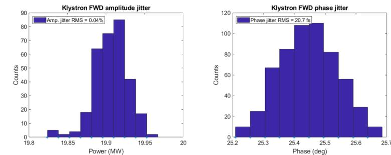
Figure 5. Measured amplitude and phase jitter of klystron output forward power. The measurements refer to 20 MW, 300 ns at 50 Hz repetition rate RF pulses.
