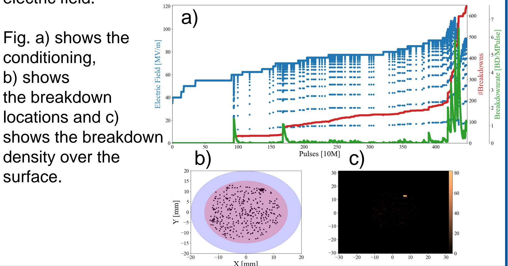
Pulses [GPulses] Additively manufactured (AM) electrodes have been tested at CERN where the top surface remains as fabricated, see Fig. a). The AM electrode was tested having 275 and 115  $\mu$ m gaps. Due to gap dependencies on the final electric field, the data has been normalized and compared with Soft Cu, which had a similar conditioning pulse time. It is observed that both electrodes reach a similar final electric field.
