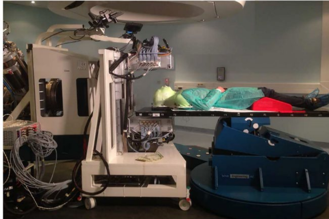
Fig. 1. Enactment of the first patient test with the INSIDE in-beam PET scanner. The system is installed in one of the CNAO treatment rooms at the working position.
