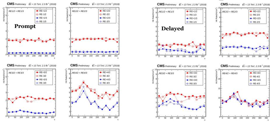
The rate of background and noise hits per layer is shown for individual RPC chambers, as a function of the azimuthal angle  $\Phi$ , at the reference LHC Instantaneous Luminosity of L =  $10^{34}$  cm<sup>-2</sup> s<sup>-1</sup>, split by the prompt component and the delayed component.
