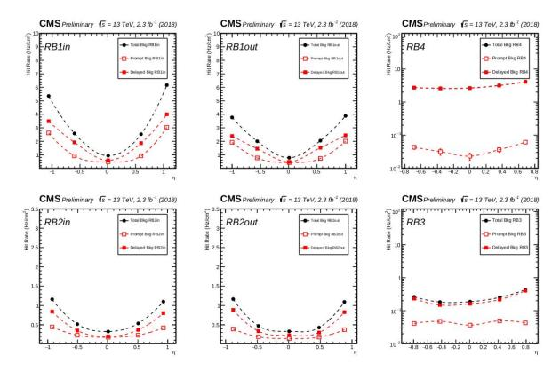
Inclusive (black circle), Prompt (red open box) and Delayed (red filled box) hit rate at instantaneous luminosity of 10<sup>34</sup> cm<sup>-2</sup> s<sup>-1</sup> in the RPC chambers in the Barrel as function of the pseudo-rapidity.
