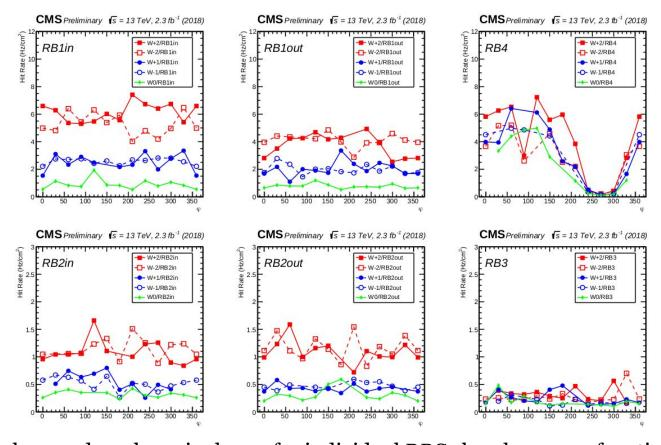
The total background per layer is shown for individual RPC chambers, as a function of the azimuthal angle  $\Phi$ , at the reference LHC Instantaneous Luminosity of L =  $10^{34}$  cm<sup>-2</sup> s<sup>-1</sup>.
