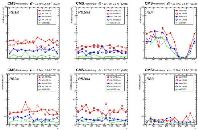
The delayed component of the background per layer is shown for individual RPC chambers, as a function of the azimuthal angle  $\Phi$ , at the reference LHC Instantaneous Luminosity of L =  $10^{34}$  cm<sup>-2</sup> s<sup>-1</sup>
