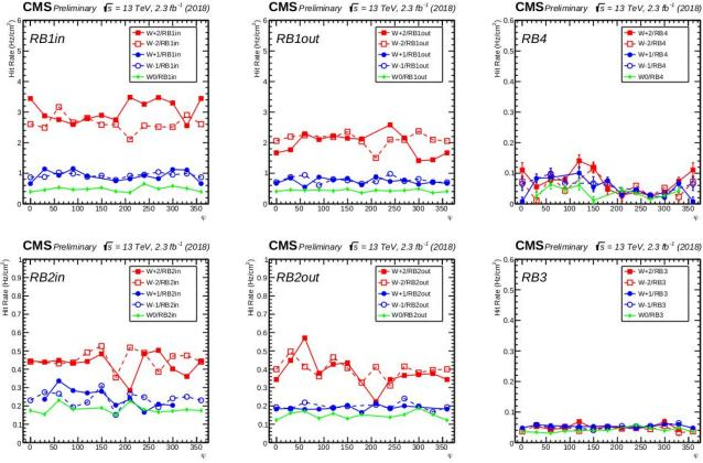
The prompt component of the background per layer is shown for individual RPC chambers, as a function of the azimuthal angle  $\Phi$ , at the reference LHC Instantaneous Luminosity of L =  $10^{34}$  cm<sup>-2</sup> s<sup>-1</sup>
