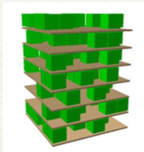
(much smaller) 90 \sim 1 \times 1 \times 1 \text{ cm}^3 scintillators
