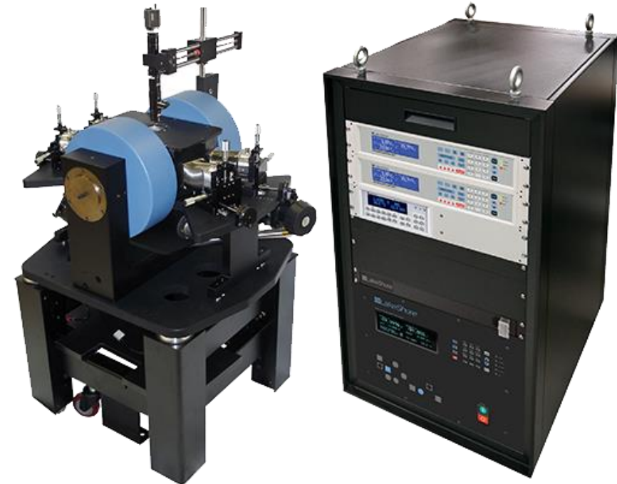
Lakeshore EMPX-HF Cryogenic RF probe station (8 K, 0.5 T and 70 GHz)
