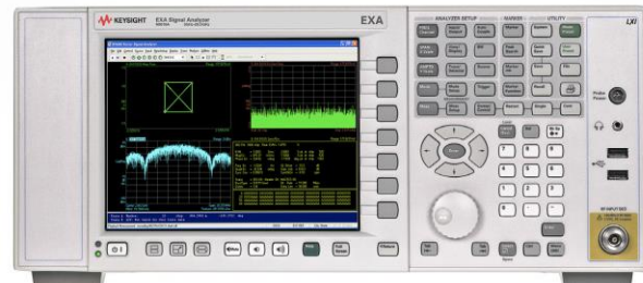
Agilent MXA N9010 spectrum analyzer, 10kHz-26.5GHz
