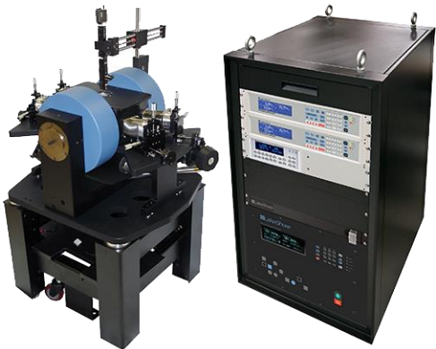
Lakeshore Cryogenic RF probe station (8 K, 0.5 T and 70 GHz)
