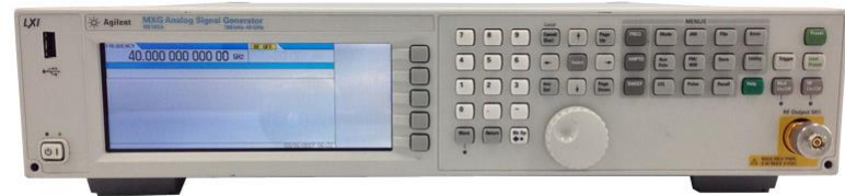
Agilent MXG N5183A signal generator, 100kHz-20GHz
