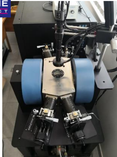
Lakeshore EMPX-HF Cryogenic RF probe station (8 K, 0.5 T and 70 GHz)
