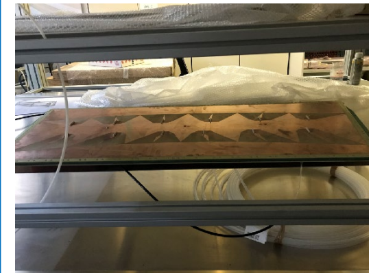
Largest \mu RWELL prototype ever built in Lab -1 in Bologna is operational with HV, LV, electronics, DAQ
