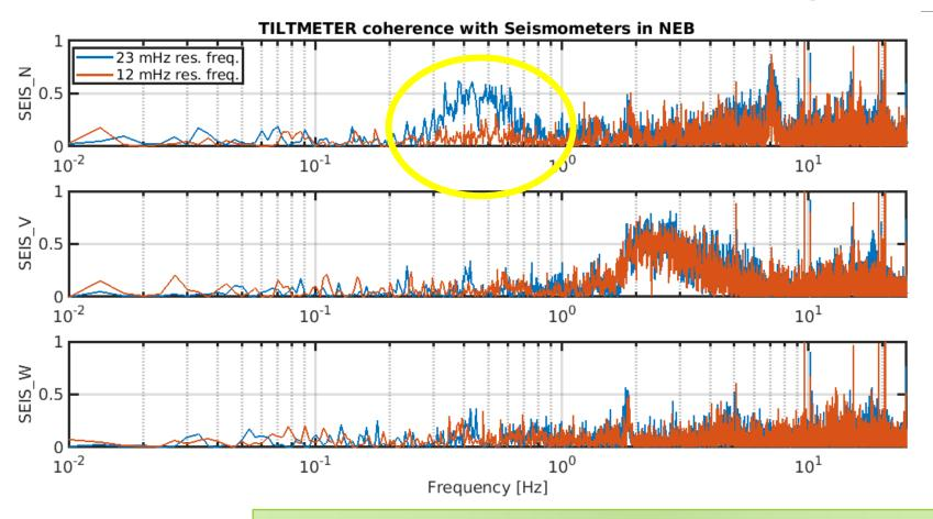
After center of mass raising, coherence with the seismometer measuring accelerations in the same direction of tiltmeter beam is highly reduced (for comparable microseismic and wind conditions)
