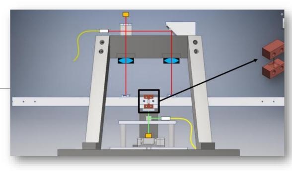
Tiltmeter arm is suspended through **Cu-Be flexible joints**, **100μm x 500μm in section**, very similar in design to LIGO tiltmeters (*Venkateswara et al., 2014*) which allow to keep **the resonance frequency below 20 mHz**
