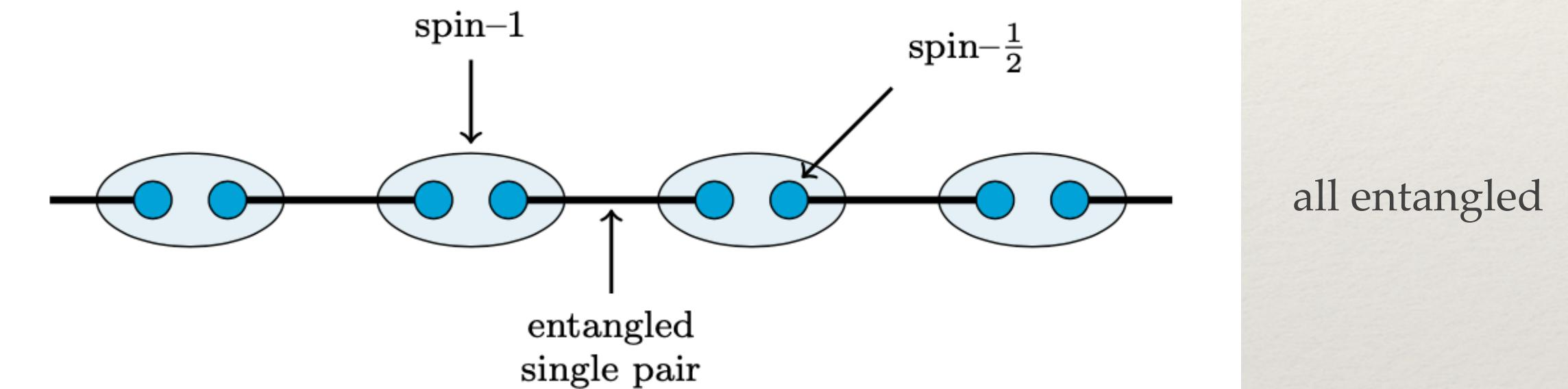
Figure 2. Entangled pair structure of the AKLT's ground state in the VBS representation: each valence bond represents a singlet state (thick black); every site, represented by an oval, contains two spin-1/2 particles (blue dots).
