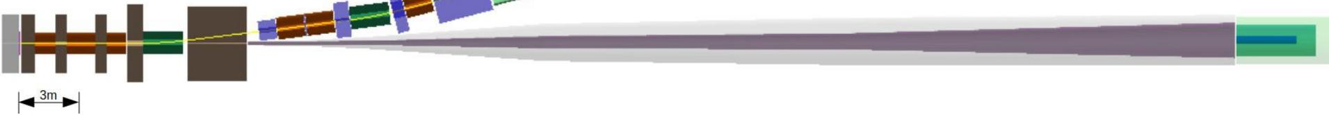
**Large bending angle of 14.8°:** better collimated beam + reduced muons background + reduced  $\nu_e$  from early decays;
