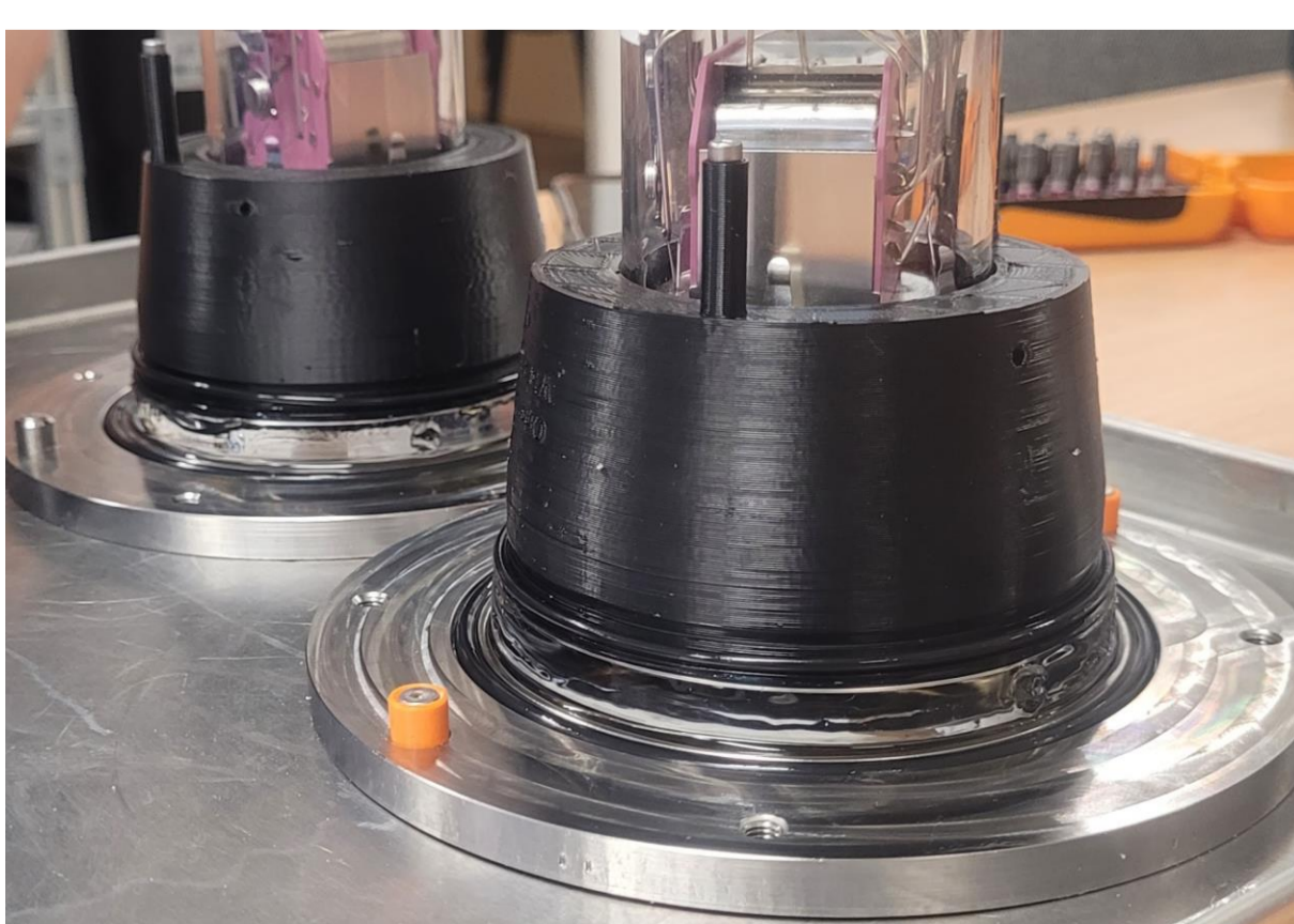
Gelled PMTs on bottom molds after top mold removal.
