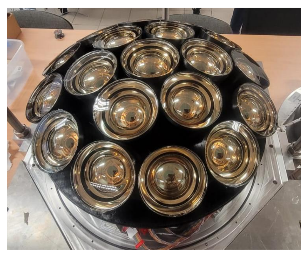
Matrix with 19 gelled PMTs before lowering acrylic cover.
