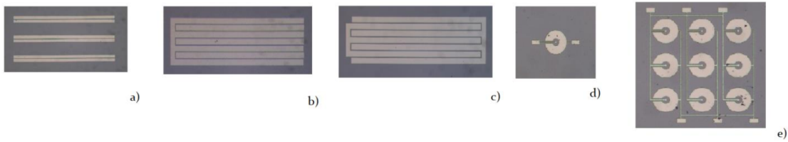
Figure 7. Lateral diode configurations: (a) strip detector, (b) comb and strip detectors (the comb is p-doped whereas the strips are n-doped), (c) double comb detector, (d) circular device (the central electrode is n-type whereas the external electrode is p-type), (e) 3 × 3 array of circular detectors.
