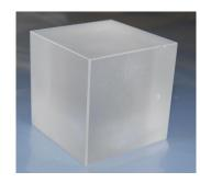
**988 detectors** of Tellurim oxide TeO<sub>2</sub> ( $Ov\beta\beta$  of <sup>130</sup>Te) for an overall **effective mass of 741 kg** !
