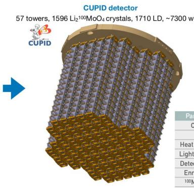
57 towers, 1596 Li<sub>2</sub><sup>100</sup>MoO<sub>4</sub> crystals, 1710 LD, ~7300 wires
