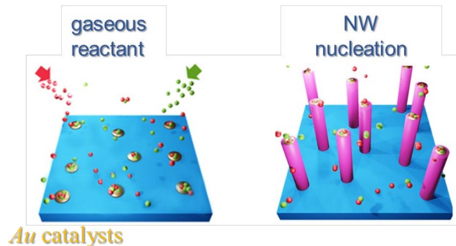
VLS: self-assembly process, catalyzed by metal nanoparticles pre-deposited on the substrate. A liquid metal/semiconductor alloy is formed. The droplet incorporates the semiconductor precursors until supersaturation. Above supersaturation, the semiconductor starts to nucleate and precipitate, giving rise to the NWs growth.
