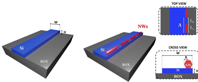
A polarization converter based on InP NWs integrated in a standard Si-waveguide was investigated. In particular, NWs having lengths  $L_a$ , are placed on the edge of a Si waveguide, at a distance  $L_b$  one from the other. According to the results of FDTD simulations, a very low number of NWs ( $N < 6$ ) is sufficient to convert the polarization of the propagating beam by 90%. Kaplan E, et al., Nanomaterials 2022, 12, 2438
