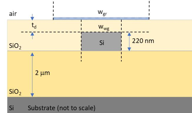
Graphene nanoribbon placed on top of a Si waveguide absorbs TE and TM modes differently. The device works switches behaviour between TE-pass or TM-pass polarizer depending on waveguide width. Cammarata S., Fontana A. et al, in press on Materials
