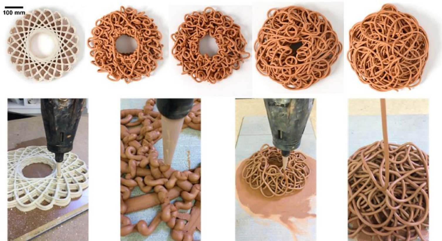
Fig. 3. Repeating pattern design with different climbing angle parameters. Leftmost- the most moderate climb with 0.01^\circ constant climbing angle. Rightmost - the steepest climb with an angle of 2^\circ . During the printing the machine tool head is way up and the clay just pulled along.
