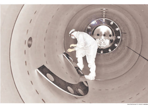
A scientist installed a baffle in 2010 to control light in the Laser Interferometer Gravitational-Wave Observatory in Hanford, Wash.
