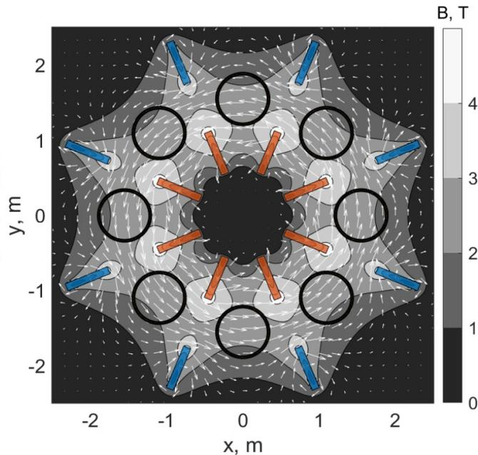
Magnetic field and load line of the conductor for BabyIAXO
