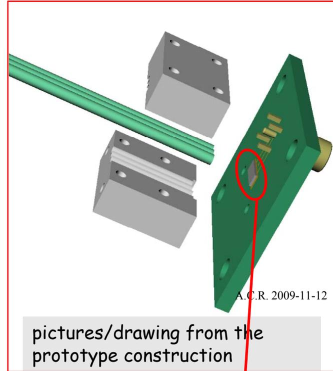
SuperB IFR : the scintillating bars are equipped with wavelength shifting fibers (3 for each bar in the prototype), which are then coupled to a SiPM device by means of precisely machined plastic supports.
