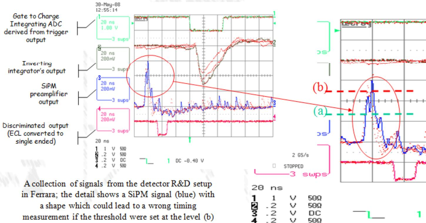
A collection of signals from the detector R&D setup in Ferrara; the detail shows a SiPM signal (blue) with a shape which could lead to a wrong timing measurement if the threshold were set at the level (b) shown in the detail.
