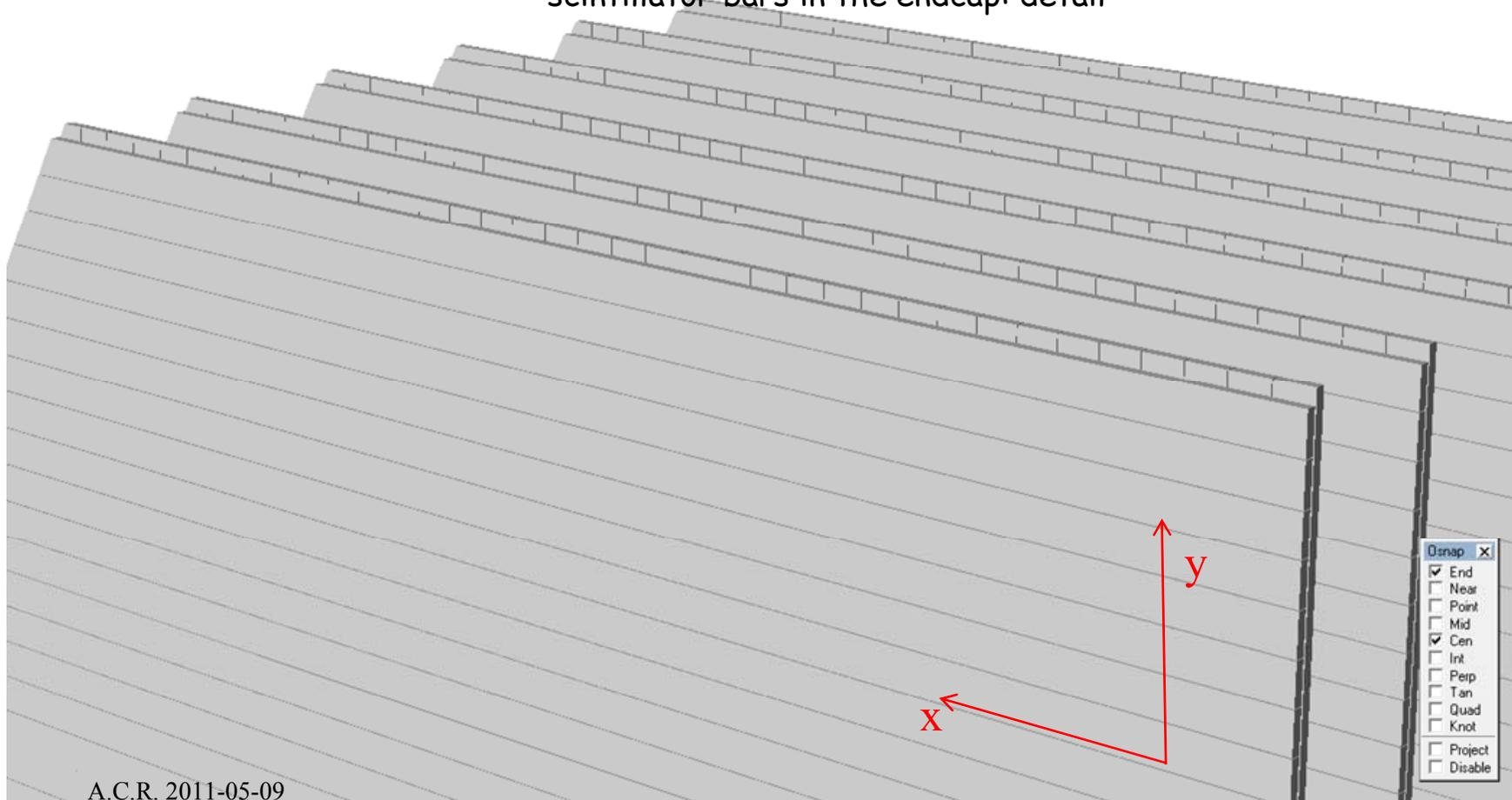
SuperB IFR: the endcaps are equipped with scintillating bars of about  $4 \times 1$   $\text{cm}^2$  cross section which are assembled orthogonally and inserted in the iron gaps. Each bar is **READ OUT BY SiPM AT ONLY ONE END.**
