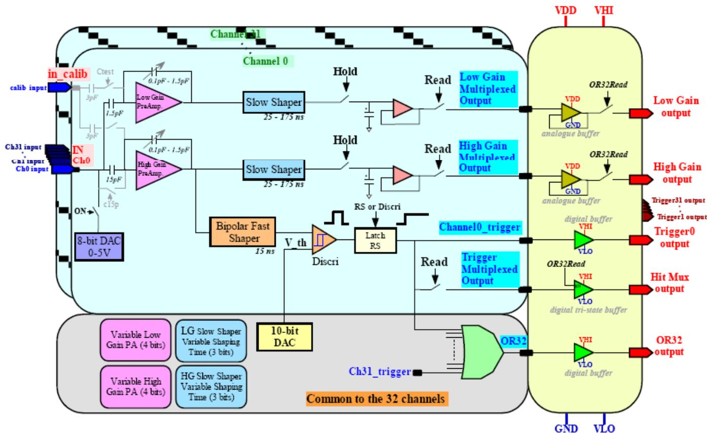
It has an individual trigger output for each of 32 channels plus 32 individual bias setting DACs and a common threshold setting DAC.
