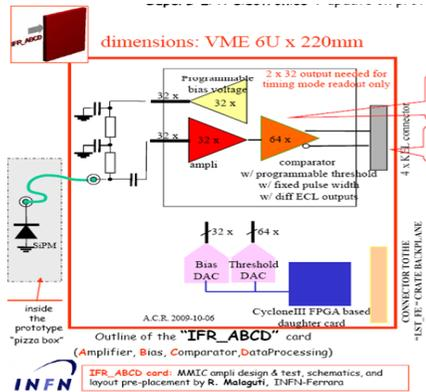
The "IFR\_ABCD" has proven to be a flexible and reliable design, easy to adapt to "p-on-n" as well as "n-on-p" SiPM devices. Its on board microcontroller allows for stand -alone operation and its amplifier monitoring outputs make the "IFR\_ABCD" a good SiPM characterization tool.
