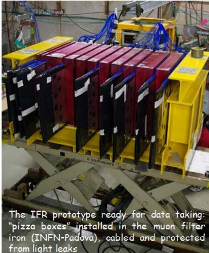
The IFR prototype ready for data taking: "pizza boxes" installed in the muon filter iron (INFN-Padova), cabled and protected from light leaks
