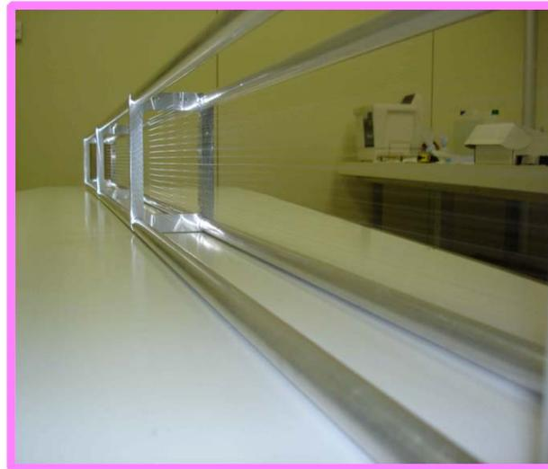
**Guard wires ensure very good linear charge and reconstruction homogeneity on all cells**
