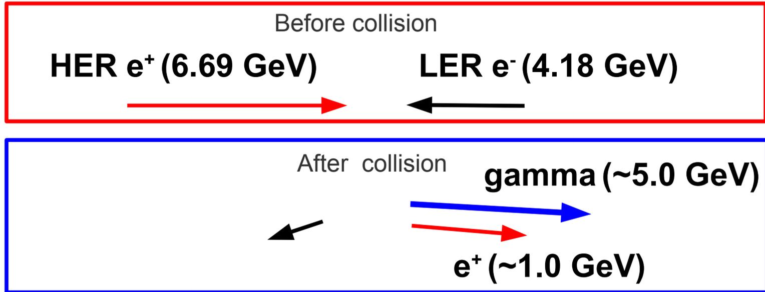
High energy gammas (5 GeV) produced via radiative Bhabha process by positrons go straight and hit the bending magnet  $\sim 10$ m away from IP, while  $\sim 1$  GeV positrons get a kick from the nominal trajectory and hit the beam pipe 1 m away from IP. This create EM showers which then affect the FTOF detector.
