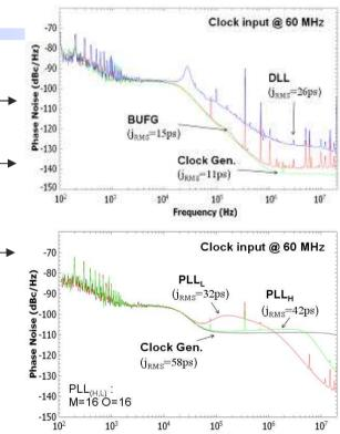
DLL can nearly double the internal jitter
