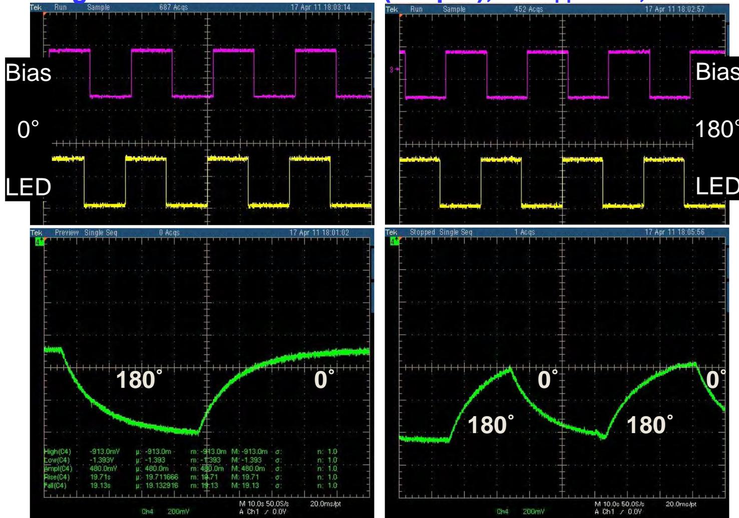
**500mV/40seconds = 12.5 mV/s = 0.125 pC/s (Capacitance = 10 pF)**
