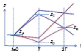
FIG. 1 (color online). Mach-Zehnder clock or atom interferometer. Two otherwise freely falling clocks (or halves of an atomic wave packet) receive momentum impulses that change their velocity by  $\pm v_0$ . The dashed lines indicate trajectories without gravity.
