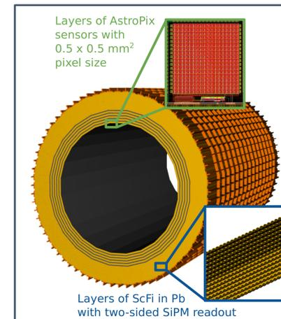
Layers of AstroPix sensors with 0.5 x 0.5 mm<sup>2</sup> pixel size
