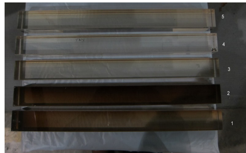
Figure 6 The lead glass blocks used to monitor the radiation dose after the C16 was placed at 10^\circ and there was 20uA beam on the 15cm LH2 target. Block 1 was placed parallel to the C16 along the beamline side of the C16. Block 1 has damage at the front (left side of photo) and along the side. Block 2 was placed in front of the C16 and perpendicular to the front face. Blocks 3,4 and 5 were located at different locations on the spectrometer platform that was near 30^\circ . These blocks show only moderate damage.
