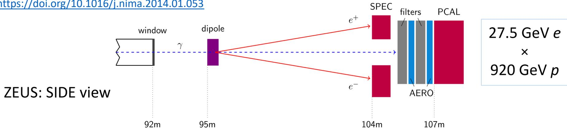
**Fig. 2.** The layout of the luminometers in the ZEUS experiment. The IP was on the left side in the ZEUS detector. A dipole magnet just downstream of the beam-exit window deflected electrons originating from converted photons to the two electromagnetic calorimeters of the spectrometer SPEC. PCAL denotes the photon calorimeter and filters the carbon absorber blocks. AERO are Cherenkov counters not used for the luminosity measurement.
