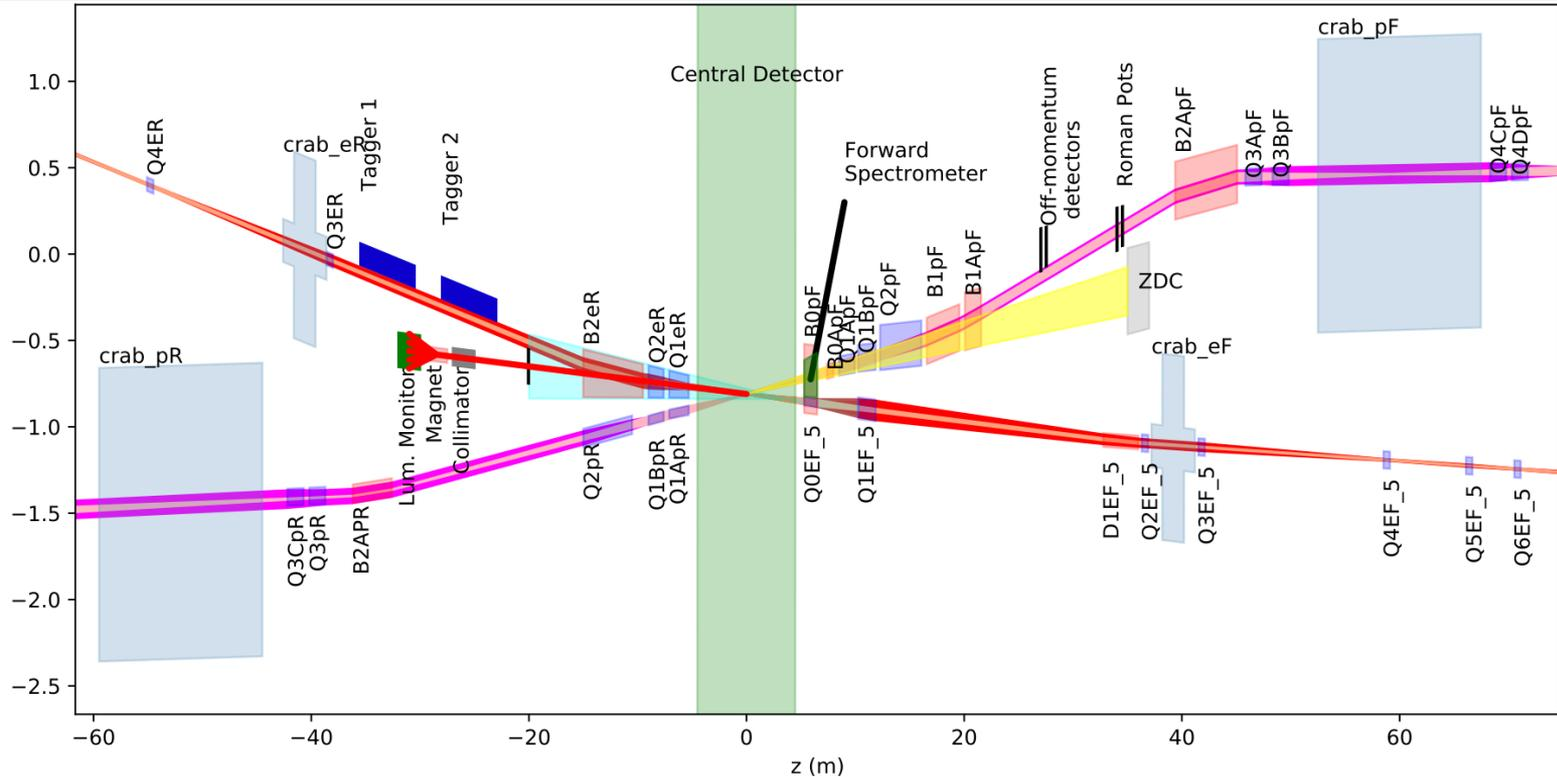
Provisions have been made in the EIC *Interaction Region* designs for the luminosity measurements using bremsstrahlung, as well as for very forward electron detectors (photoproduction taggers)
