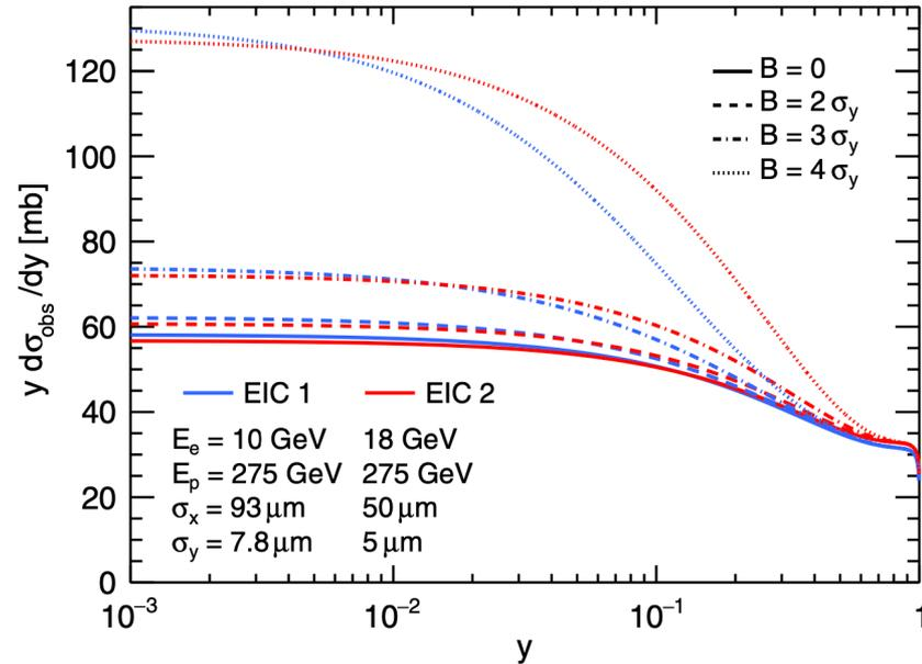
FIG. 4. The predicted spectra of  $ep$  bremsstrahlung at the EIC for several vertical beam displacements. The standard Bethe-Heitler cross section  $d\sigma_{\text{BH}}/dy$  is modified due to the beam-size effect and beam displacements  $B$ . The effective cross sections (multiplied by  $y$  for better visibility) are shown for two cases of electron-proton collisions at the EIC—the corresponding beam energies and Gaussian lateral beam sizes at the interaction point are listed.
