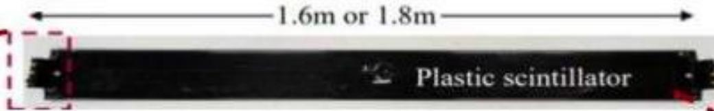
160 Eljen EJ-200 plastic scintillator, 0.6cm thick, 1.5-1.8m long, arranged overlapping in panels
