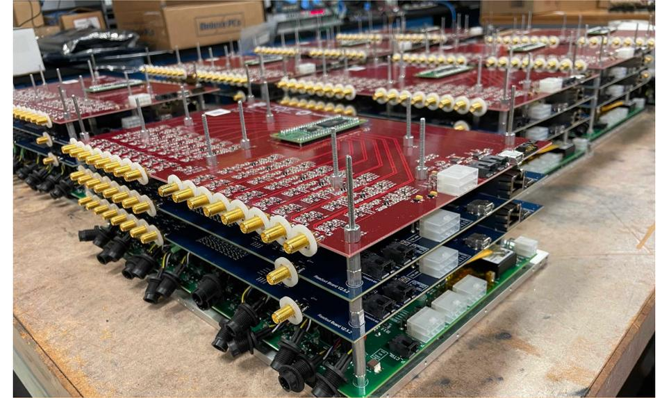
TOF readout-and-trigger electronics stack, contains 2 readout boards, local trigger board, and power board
