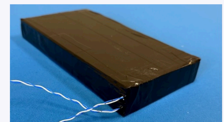
BGO scintillators with SiPM readout
