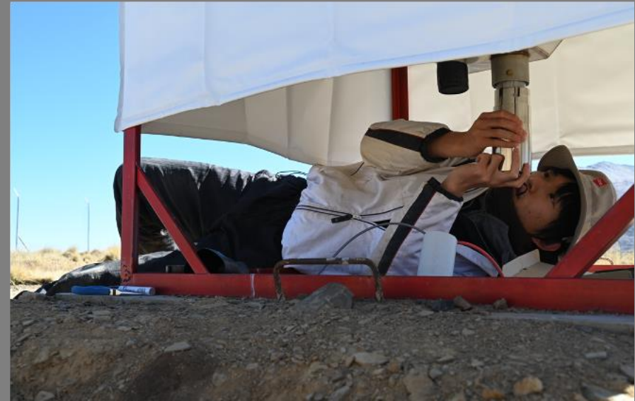
Installation of PMTs
